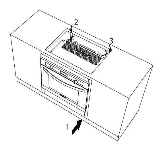
STEP 3 - Open the oven door and screw 4 screws
